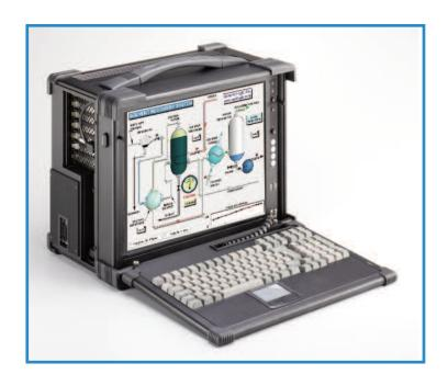
The Guardian II Series are robust lunchbox portable computers built using heavy duty metal to provide a tough, go-anywhere unit ideally suitable for harsh/severe environments and mission critical applications. With 2 drive bays and up to 4 or up to 7 full length expansion slots (depending on the model), the Guardian II can be freely configured with other uniquely designed expansion cards for most applications.
